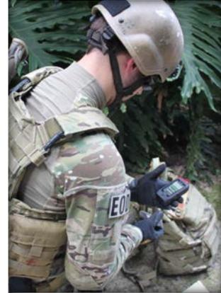
The SEEKERe Explosive Detection System by DetectaChem is the world's smallest, most rugged, automated explosive detection system. The system is comprised of a dedicated handheld electronics package with a consumable sample swipe card. The MobileDetect detection system is an even more inexpensive option for drug and explosive detection and pairs a small swab pouch with a mobile phone-based application that can be run on any first responder or border patrolman's phone.
